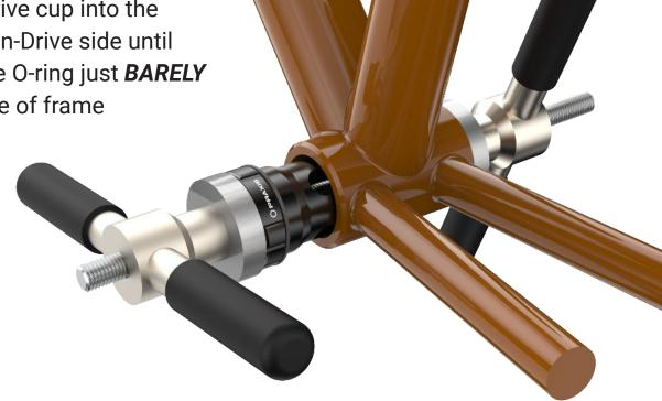
2 Start threading the Right/Drive Cup in CLOCKWISE with your M30 BB tool.
