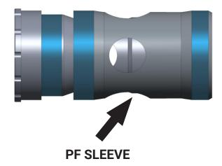
**Grease** both ends of the PF sleeve contact surfaces
