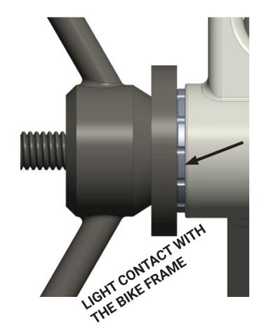
2 Start threading the **Right/Drive Cup** in **CLOCKWISE** with your M30 BB tool. As it threads in, you will feel friction build as the Orange Rubber Collet expands inside the frame. **This is normal. TURN Right/Drive Cup UNTIL IT STOPS, but do not fully tighten**
