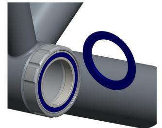
See next page to find correct Dust Covers for your crank. Lightly grease underside of Dust Covers and place them over bearings with Praxis logos facing outward. Now you can install the crank
