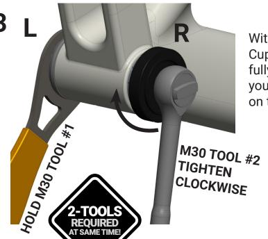
With 2nd M30 BB tool, hold Left/Non-Drive Cup in place while you tighten Drive cup fully. The 2nd tool gives you leverage so you feel when the Drive cup bottoms out on the Non-Drive cup
